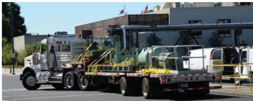
The new chassis dyno had to be disassembled in California and trucked across the country to ESW America's headquarters in Montgomeryville, Pa. The chassis dyno is capable of handling vehicles ranging from passenger cars to Class 8 trucks, buses and other single- or tandem-axle-drive, heavy-duty vehicles, with inertia simulation from 2000 to 85,000 lb.
