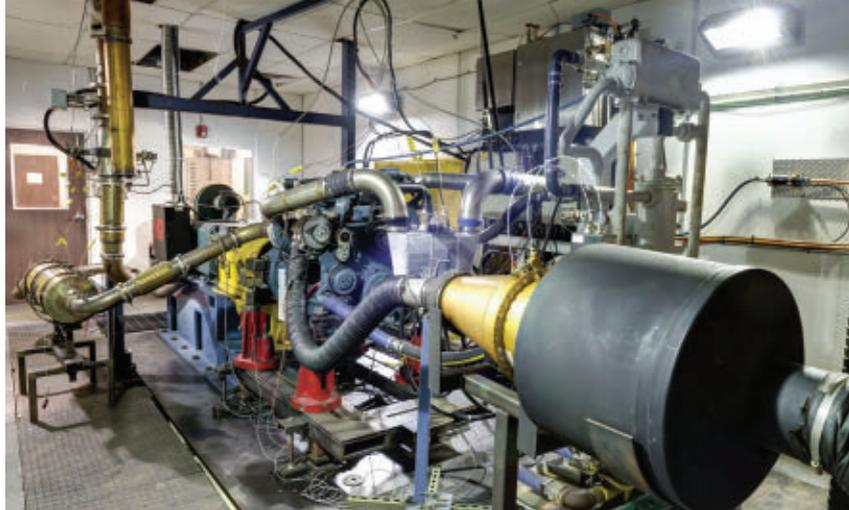
ESW America has eight test cells at its Montgomeryville, Pa., headquarters. The company can perform research and development and certification test programs for motorcycles, UTVs, ATVs, small off-road engines and heavy-duty diesel engines up to 1000 hp.
